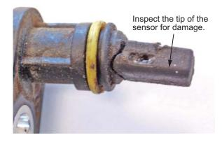
If the tip of a sensor has any damage, do this:
