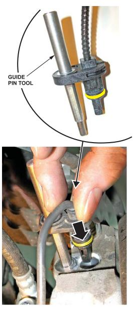
8. Insert the ABS wheel speed sensor and the guide pin into the knuckle assembly.
