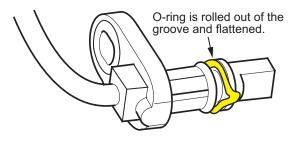
If a sensor O-ring is pinched or damaged, do this:
