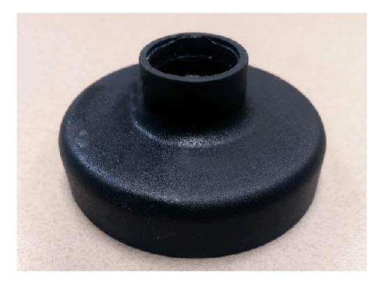
Use the following steps to inspect the steering gear input shaft for the presence of an "Umbrella Seal". If no seal is installed, it will be necessary to replace the steering gear.
