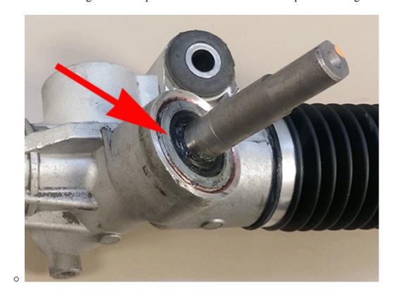
If the seal **is not** installed, proceed to the section below.
